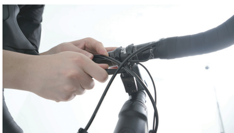
If you have an electronic shifting system, remove the three cables from the junction box (using the appropriate tool) before removing the handlebar. Failure to do so will likely cause damage.
