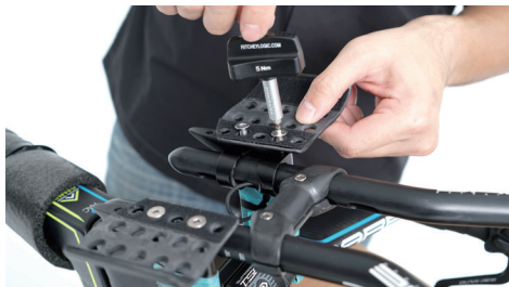
Once an appropriate position has been found, tighten the B5/B6 without fully tightening since further adjustment will be required later.
