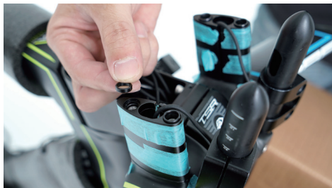
Align the oval plate with the riser and then position a C2 in the two indented holes of the oval plate.
