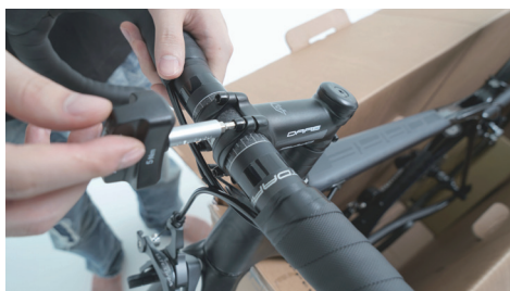
Loosen the stem face plate, remove the handlebar and secure the face plate once more (enough to hold it in place and no more).
