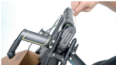
Select the M2 and release the screws on the stem cover.
