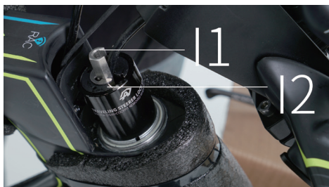
Insert the supplied I1 into the I2 within the DARE steerer tube lock spacer I3 .
