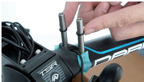
Fit a C1 to each bolt before fitting the riser kit.
