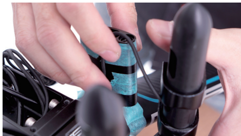
Position the riser kit onto the mandrel bolts on the handlebar (The riser kit is an irregular oval. Ensure the fat end faces forward and the narrow end backwards). Pull the gear cable through the riser kit and place in the center.
