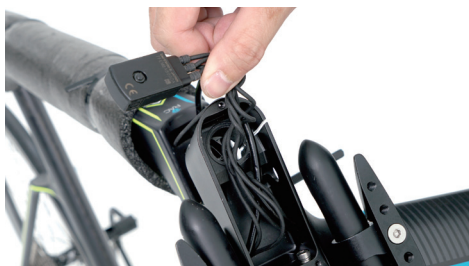
Take out the junction and wires of DI2 .
