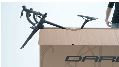
Place the bike into the EZBOX so that the rear wheel is positioned in the corrugated paper seat and the forks overhang the front of the box.
