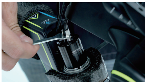
Use the supplied M1 to loosen I2 by turning counterclockwise.
