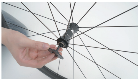
Take out the hub protection and insert it into one side of the hub.
