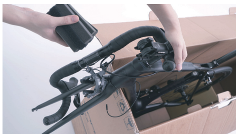
Position the handlebar as shown in the picture and use three high density foam pieces and belts to fasten the handlebar at the three locations as shown below, namely the top tube, head tube and fork.
